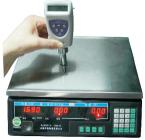
Apply a force N to the tip. When readings are almost unchanged, press the key 'MAX' to hold the reading P which should satisfy the equation below.
