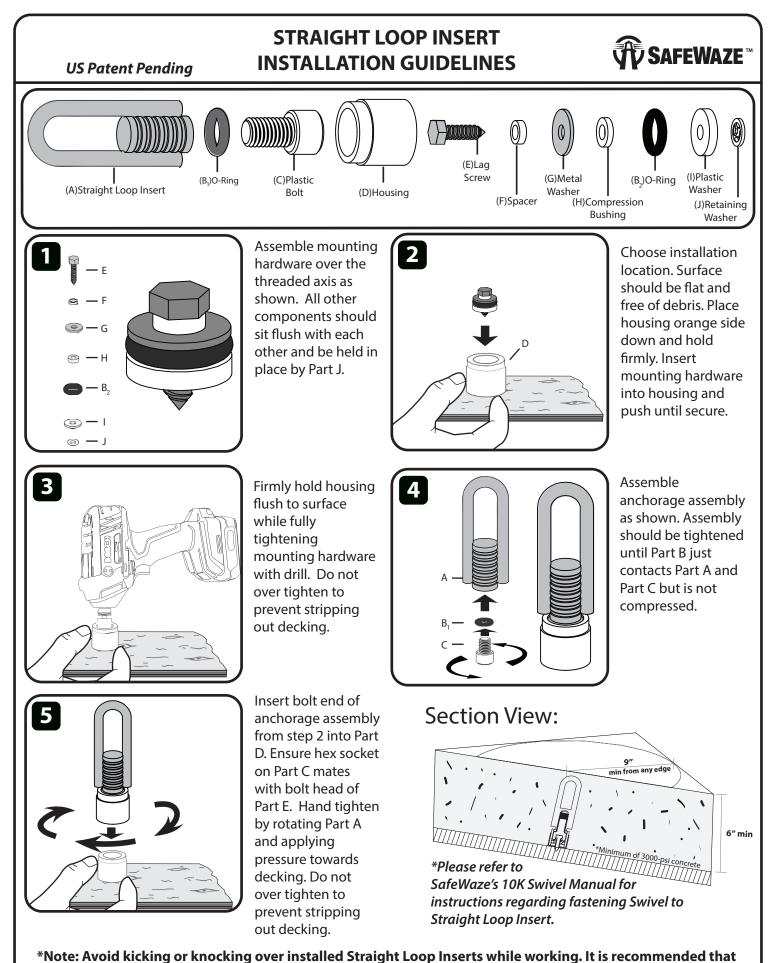
inserts are fastened to rebar by wire tie or equivalent method for additional support.
