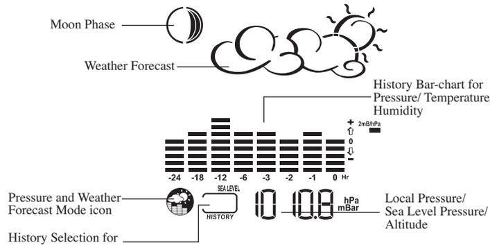
**NOTE:** An altitude display of 990, is actually 990 feet, etc. Pressure can be displayed as: "inHG" (default) inches of mercury, "mmHG" is millimeters of Mercury and "hPa/mBar" is scientific hectoPascal.
