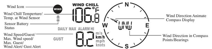
**NOTE:** The wind speed alert is set at 5 mph default and the wind gust alert is set to 7 mph default to prevent false alerts from small fluctuations.
