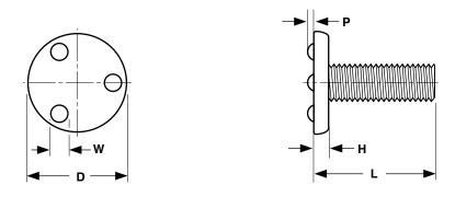
±Length of a weld stud is measured from the welding surface of the head to the end of the shank, excluding the projections.
